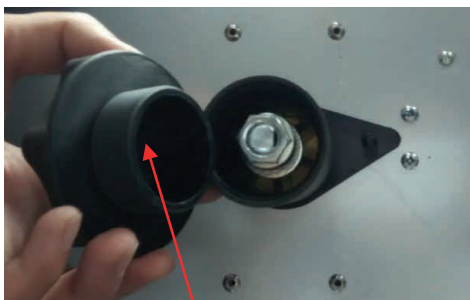
(1) Remove the spool retaining nut.
